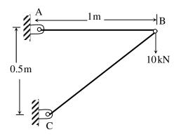
ME-GATE-2014 PAPER-02 Answer: 18 to 22 Exp: FBD of joint B  $\theta = \operatorname{Tan}^{-1}\left(\frac{0.5}{1}\right) = 26.5$   $\Sigma V = 0$   $\frac{F_{BC} \sin \theta}{F_{BC} \cos \theta} = \frac{10 \text{ kN}}{F_{AB}}$   $F_{AB} = \frac{10}{\operatorname{Tan} 26.2}$ = 20 kN.
