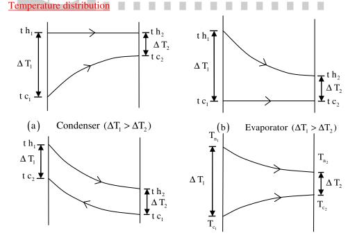
(c) Counter flow Heat Exchanger  $(\Delta T_1 = \Delta T_2)$  (d) Parallel flow Exchanger  $(\Delta T_1 > \Delta T_2)$
